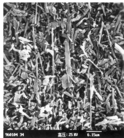
Fig. 2. SEM micrograph of oriented SiC(w)/Si 3 N 4 composites.
